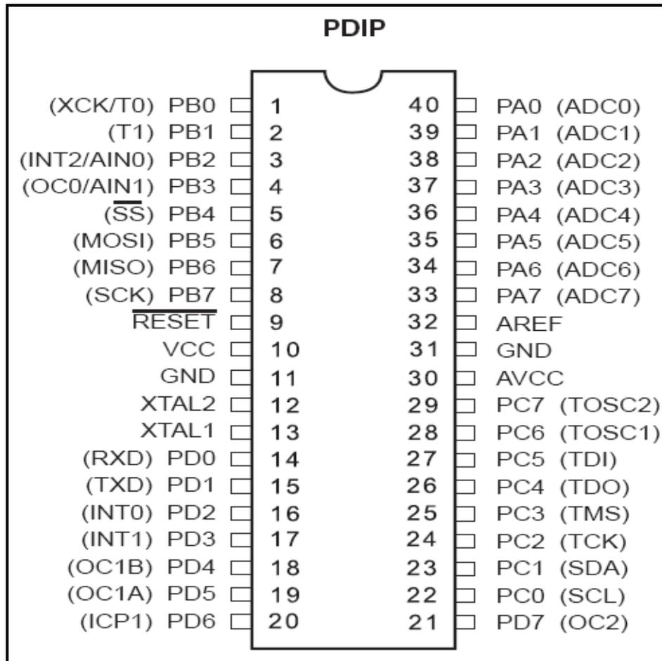
Fig (3):- Pin out of ATmega32
