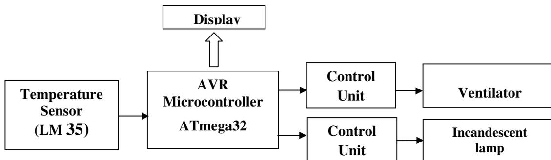
Fig (1): - Block Diagram
