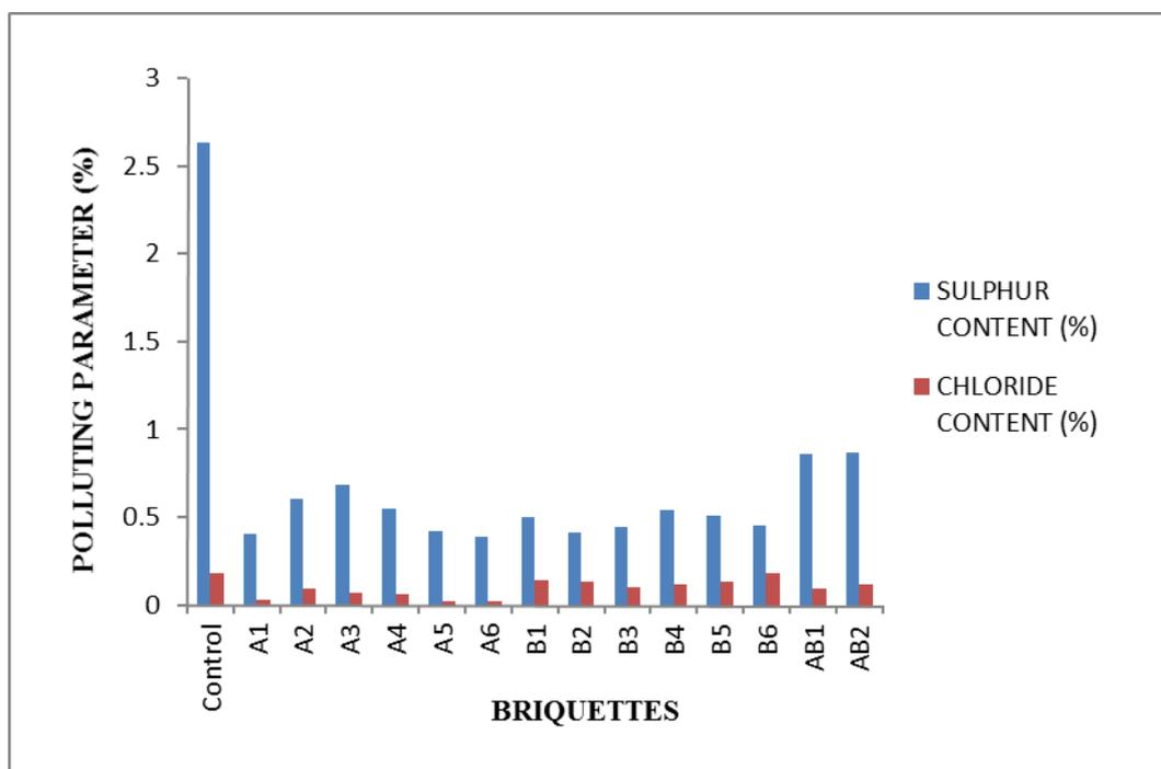
**Figure 4: Sulphur Content & Chloride Content of different Briquettes**
