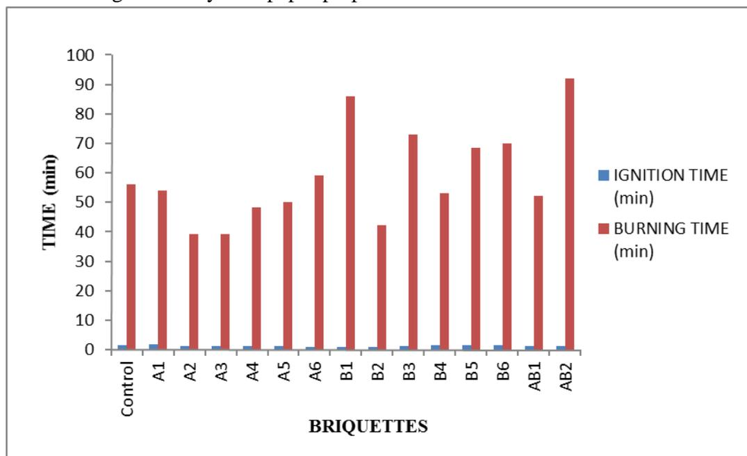
Figure 3: Ignition Time & Burning Time of different Briquettes
