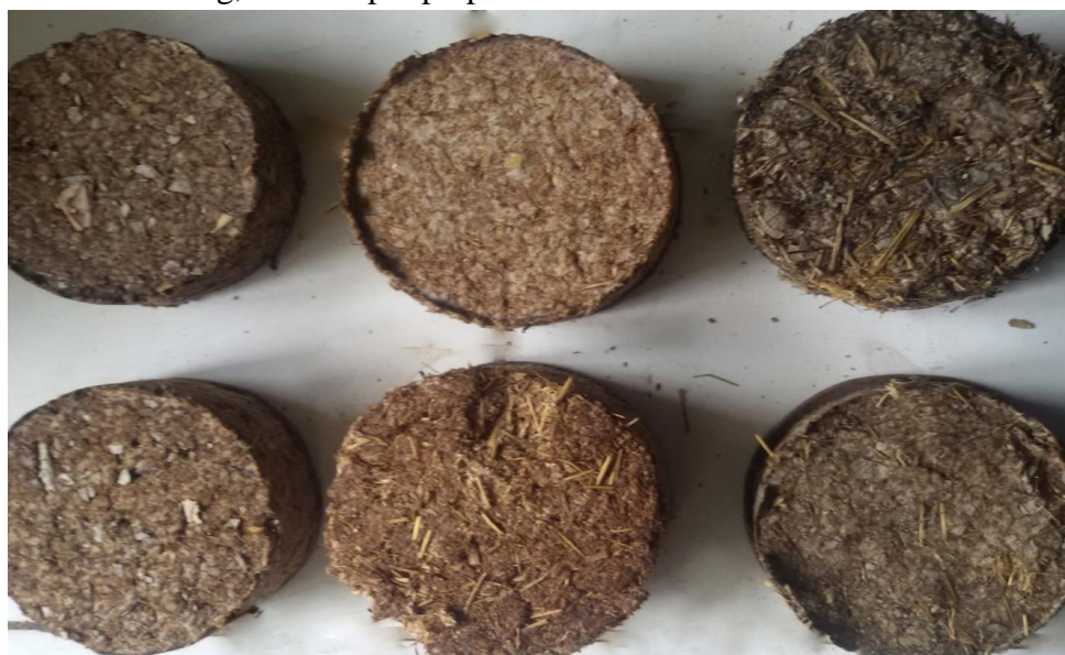
Figure 2: Produced Briquettes with different Feed stocks (dry leaves, wheat straw & saw dust) & Binders (paper pulp & cow dung)
